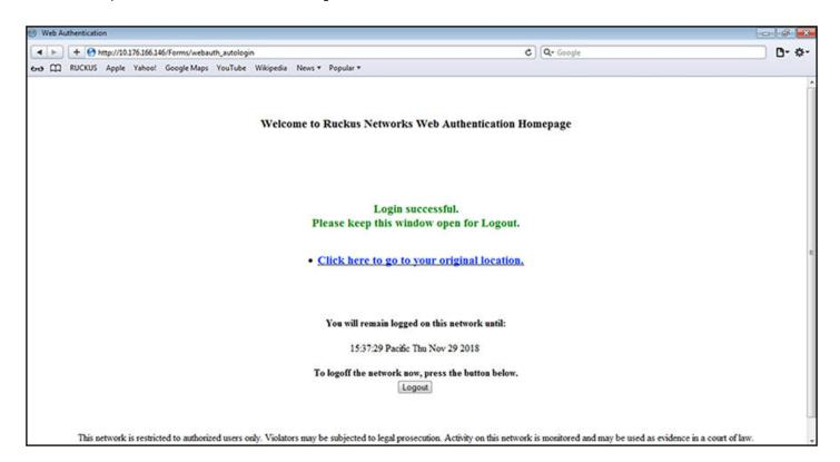
Once a host is authenticated, that host can manually de-authenticate by clicking the Logout button on the login success page. The host remains logged in until the re-authentication period expires. At that time, the host is automatically logged out. However, if a re-authentication period is not configured, the host remains logged in indefinitely.
