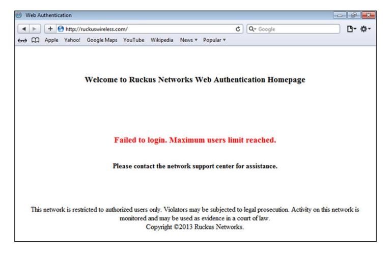
If the number of Web Authentication attempts by a user has been exceeded, the maximum attempts limit page is displayed. The user is blocked from attempting Web Authentication until either the user MAC address is removed from the blocked list (using the **clear webauth block-mac** command) or the block duration timer expires.
