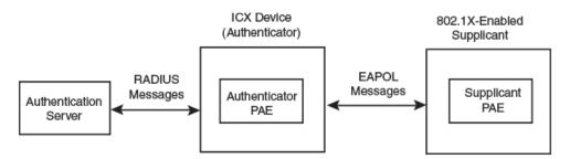
Authenticator PAE: The authenticator PAE communicates with the supplicant PAE, receiving identifying information from the supplicant. Acting as a RADIUS client, the authenticator PAE passes the supplicant information to the authentication server, which decides whether the supplicant can gain access to the port. If the supplicant passes authentication, the authenticator PAE grants it access to the port.
