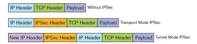
Internet Key Exchange (IKE) is used to establish an IPsec tunnel. IKE performs mutual authentication of peer devices and establishes and maintains a secure channel for communication between the devices.
