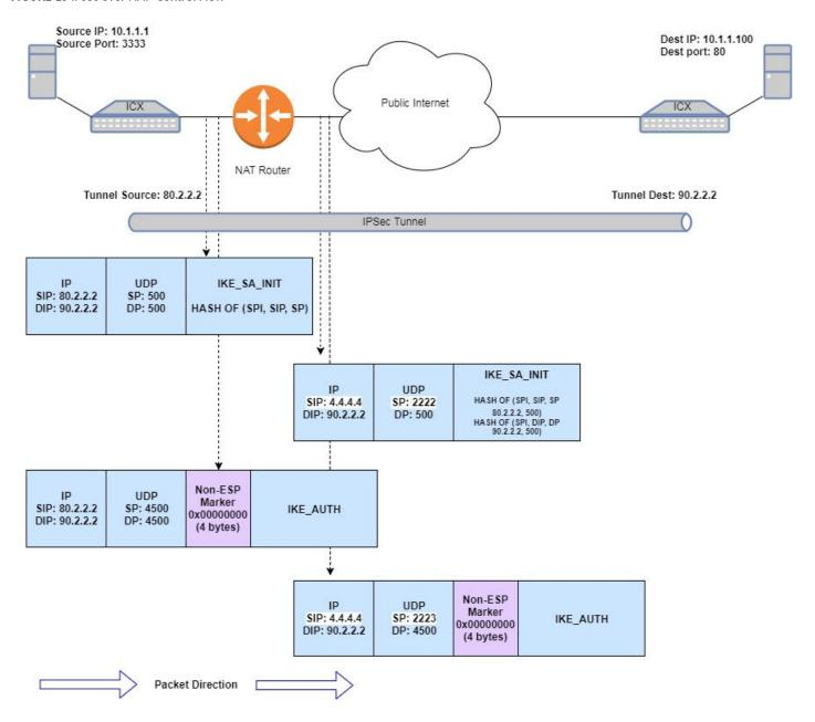
On the other side, again the hashes of IP address and port are calculated in the packet header. The re-calculated hashes are compared with the hashes received as part of the NAT-D payload. If they are different, it means the packet has undergone NAT. After this negotiation, the IPsec tunnel is established with UDP encapsulation. In UDP, both source and destination ports are set to 4500.
